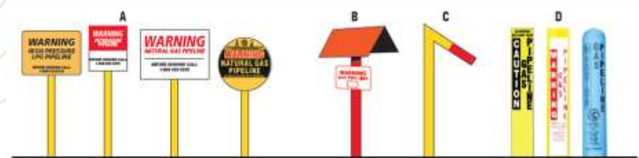
A. Located near roads, railroads and along the pipeline ROWs B. Marker for pipeline patrol plane C. Pipeline casing vent D. Painted metal or plastic posts
